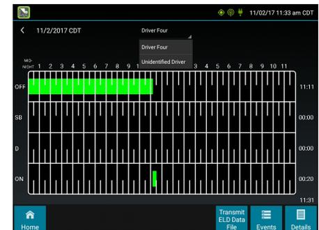
To view all unassigned unidentified driver events recorded by the device, tap the driver's name (above the grid) and tap Unidentified Driver. Use the arrows on either side of the date or swipe the screen side to side to navigate through the log history.
